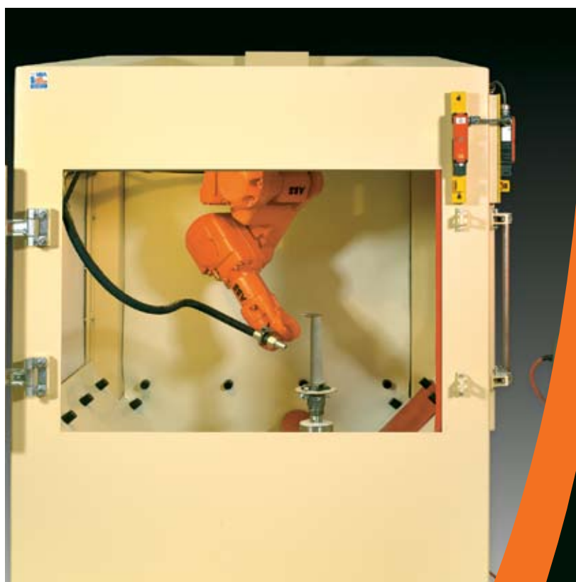
Roof mounted robot opens the work envelope to a full 360° and often eliminates the need for a seventh axis.
